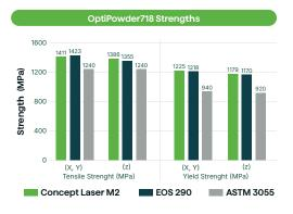
Continuum Powders offers OptiPowder Ni718 in various particle size distributions (PSD) to meet your specific manufacturing needs. Representative properties shown here are for laser powder-bed fusion (LPBF) powder PSD.
