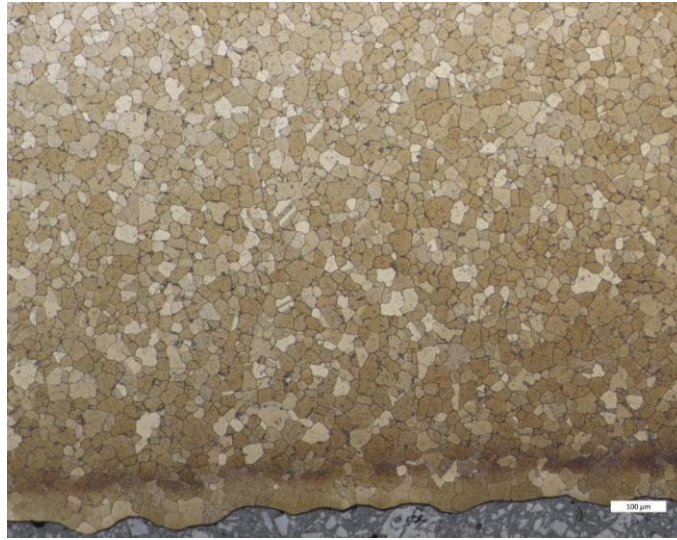
Figure 13. Process condition “HPHT+Age1000+Age800” LOM etched moclonics.
